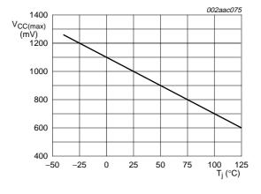
Fig 9. V<sub>CC(max)</sub> that guarantees bus release limit over temperature
