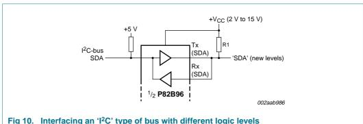
Fig 10. Interfacing an 'I2C' type of bus with different logic levels
