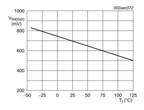
$V_{\text{IH}(\text{min})}$  at Sx changes over temperature range
