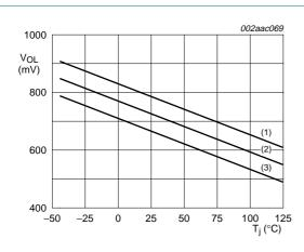
V<sub>OL</sub> at Sx typical and limits over temperature
