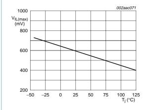
$V_{\text{IL}(\text{max})}$  at Sx changes over temperature range
